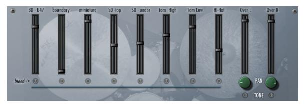
This section lets you mix the different microphone signals, control the bleed signals for the close mics, and also control the panning and tone of the overhead channels.
