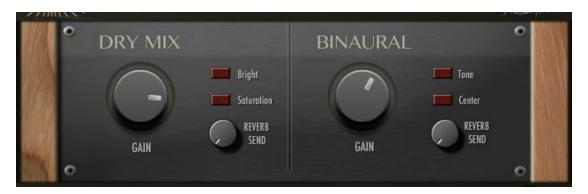
This section lets you mix the two different signal paths, add effects to each channel and send part of the signal to the master Reverb.
